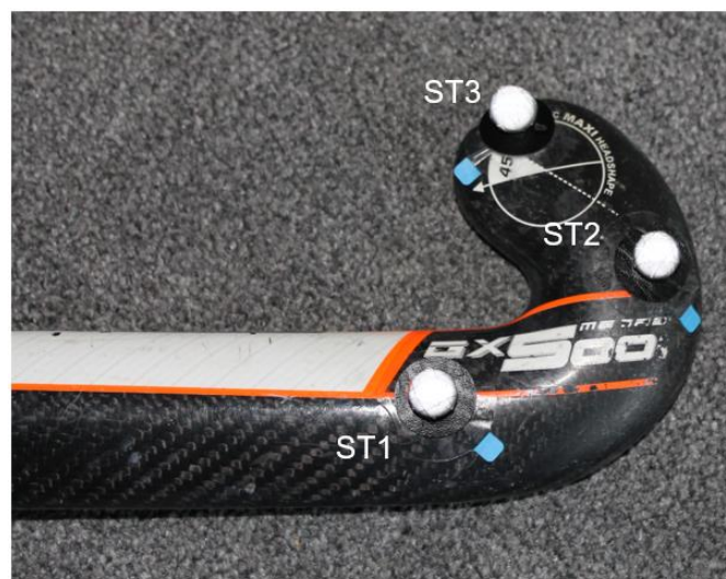
Figure 19 Static and tracking stick markers. Source: Created by the author.
