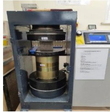
Figure 3.11: Compressive testing machine for testing of 100 mm cubes
