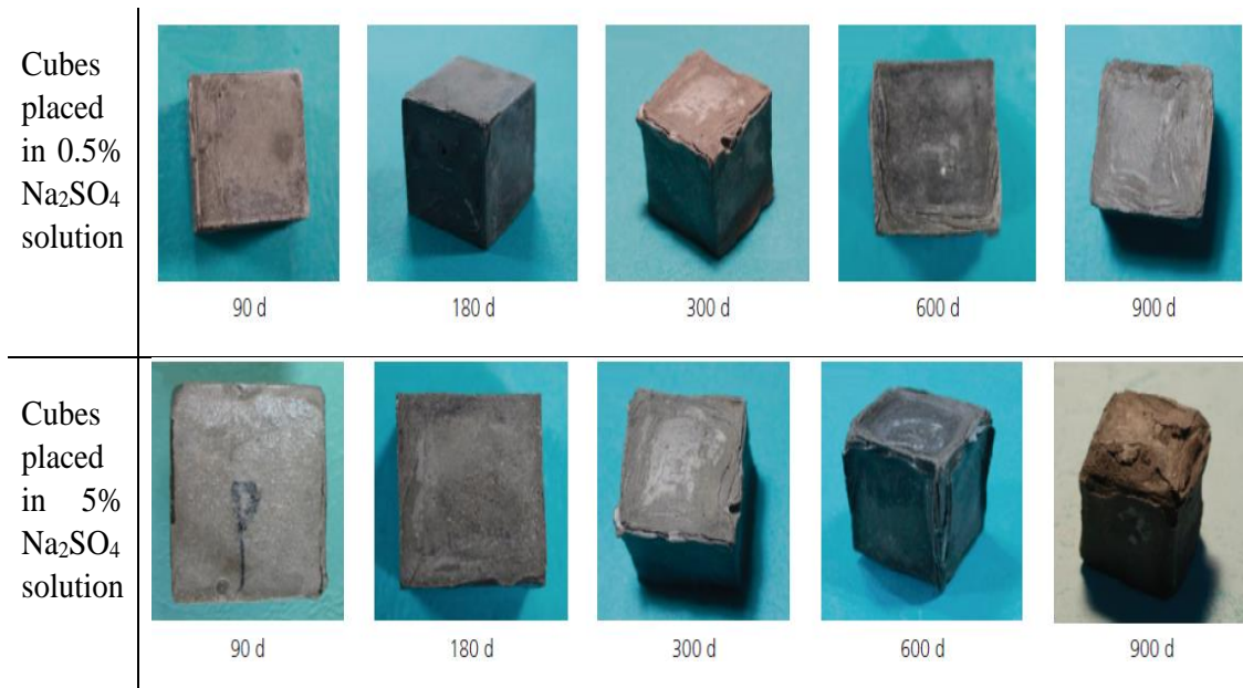
Figure 2.65: Qualitative Analysis of OPC cubes in 0.5% and 5% \text{Na}_2\text{SO}_4 solution after 900 days (Liu et al., 2015).
