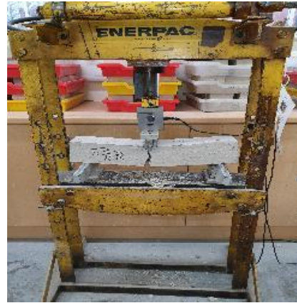
Figure 3.13: Three-point flexural strength testing of prism
