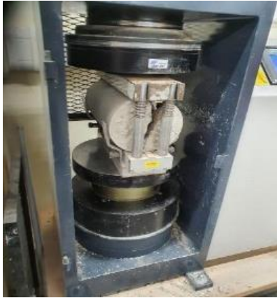
Figure 3.12: Cylinder testing for split tensile strength of concrete
