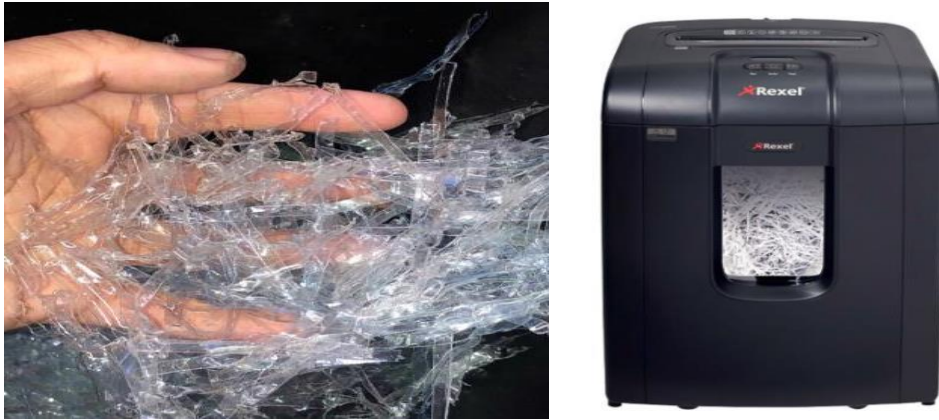
Figure 2.60: PET Bottle Fibres Shredded Using a Paper Shredder (Nadir et al., 2022a)
