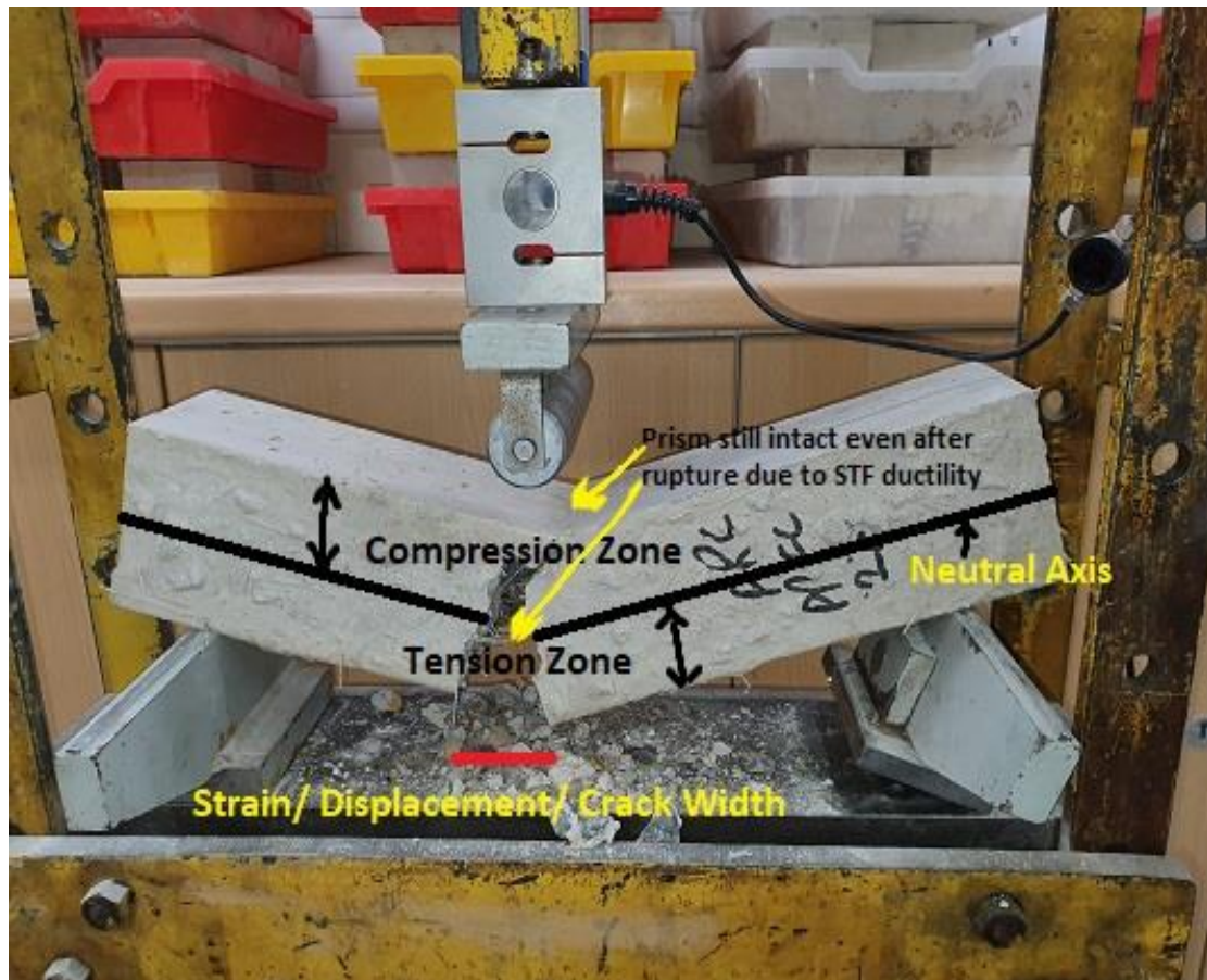
Figure 4.44: Mechanism of Post-Crack Ductility in Fibre-Reinforced Prisms During Flexural Strength Testing.
